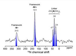
**Figure 5.** Solid-state 1D  $^{15}$ N{ $^{1}$ H} DNP–CP–MAS spectra of 100%-amine–coCOF–H without CO $_{2}$  exposure. The spectrum was acquired at 9.4 T, 8 kHz MAS, 95 K, in the presence of 16 mM AMUPol biradical in 60:30:10  $d_{8}$ -glycerol/D $_{2}$ O/H $_{2}$ O, under microwave irradiation at 263 GHz, and using cross-polarization contact times of 5 ms. Blue markings correspond to values obtained by quantum-chemical calculations (See Tables S4, S5, and S7).
